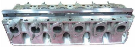
Place the ruler and check with a feeler gauge the difference, as shown.
